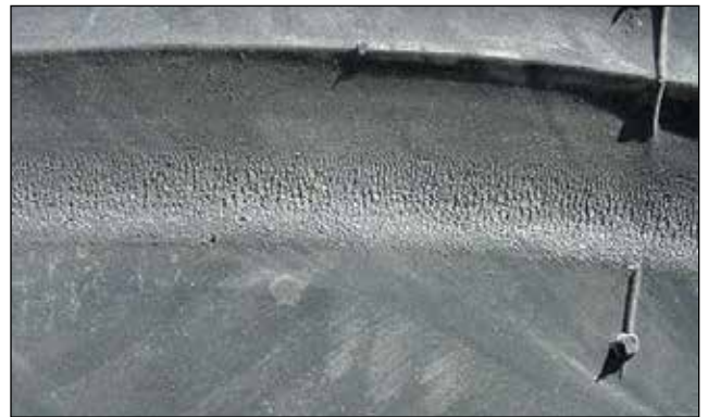
Abrasion Marks on the Sidewall
