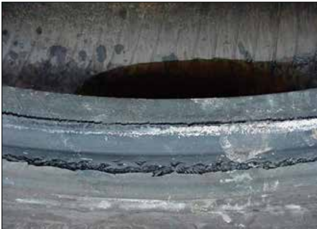
2nd Stage – Bead Splitting from Heat
