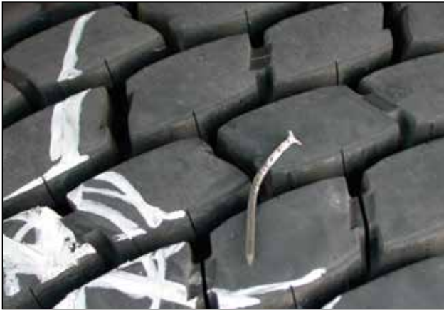
Inspect for Penetrating Objects
