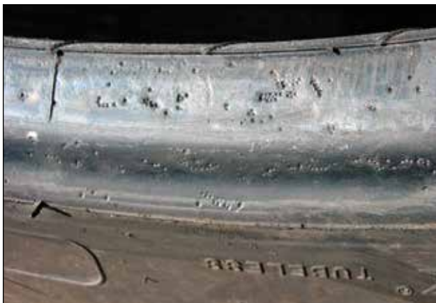
Deterioration from Foreign Matter Between the Wheel and Bead
