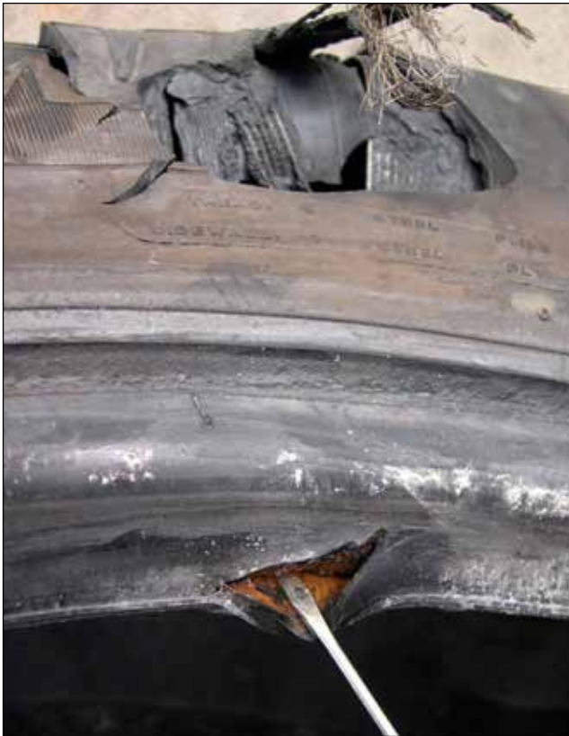
EFFECT: Sidewall Separation Due to Air Infiltration Resulting from Bead Damage CAUSE: Due to Mount/Dismount
