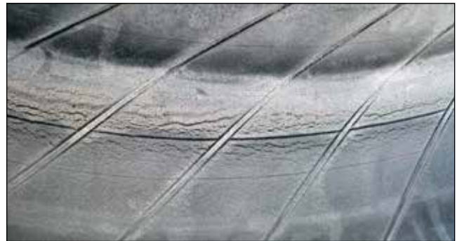
EFFECT: Inner Liner Cracking CAUSE: Underinflation
