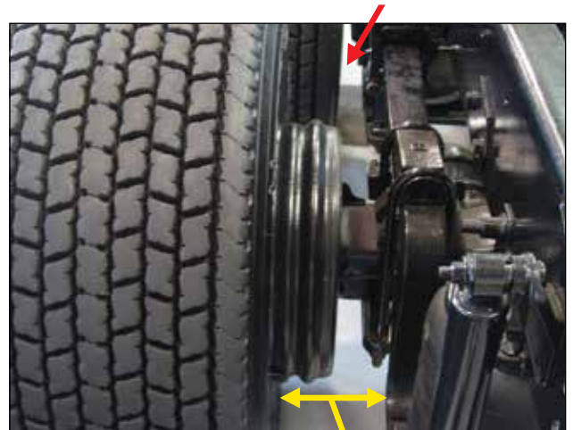
Correct Lateral Clearance
