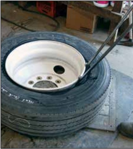
4 Be sure to start at the valve stem, not away from or opposite.
