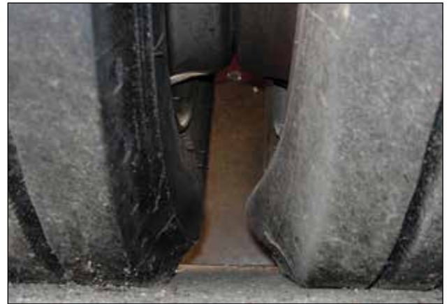
Mismatched pressure in dual position will cause the tires to rotate at different revolutions per mile resulting in irregular wear and tire damage.
