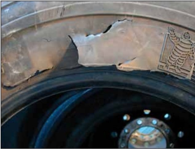
EFFECT: External Rubber Damage CAUSE: Severe Impact
