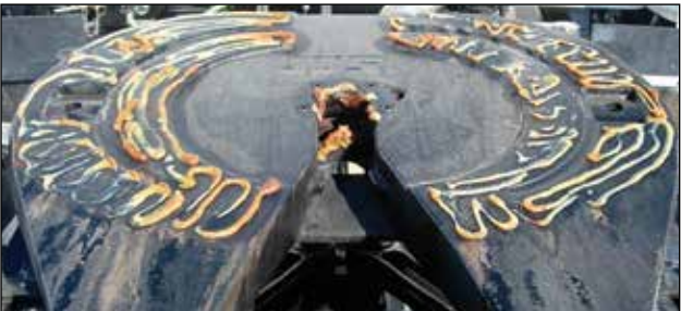
Proper Amount of Lubrication
