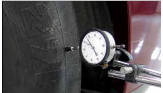
Measuring Lateral Runout on Outside Shoulder
