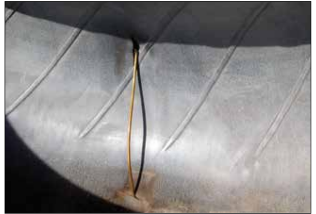
Example of sidewall penetration that damaged interior at crown. Road hazard damages should always be inspected on the inside and not repaired from the outside.
