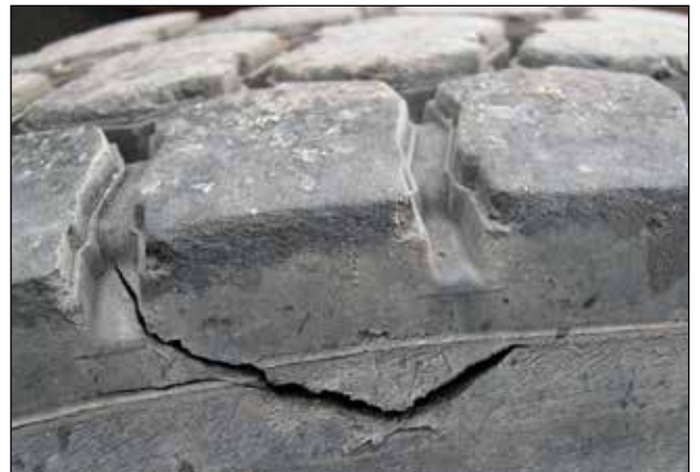
Sidewall Area Damage
