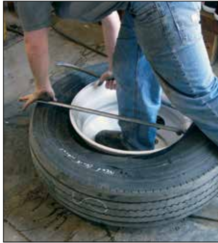
5 Step forward into the drop center, laying the bars down.
