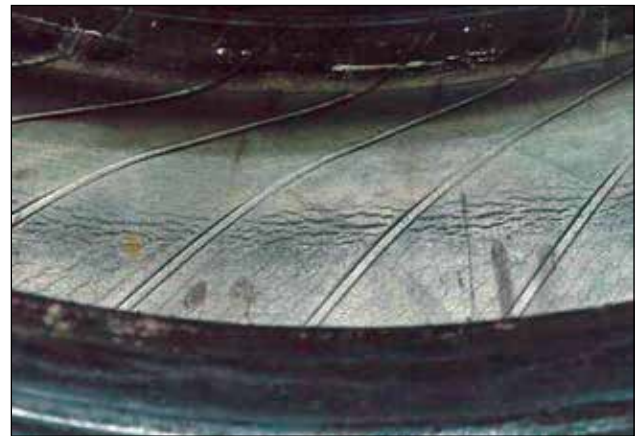
Sign of Run Flat Damage – Interior
