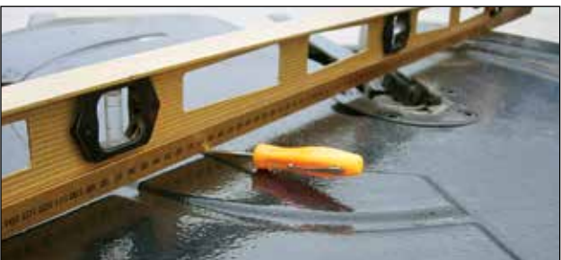
Distortion of the 5th Wheel
