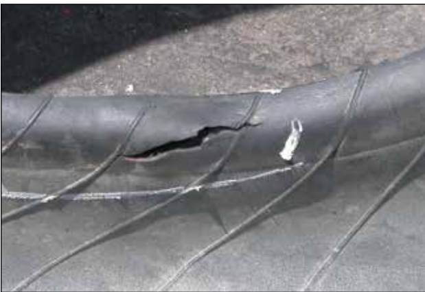
Bead Damage Caused by Mounting/Dismounting
