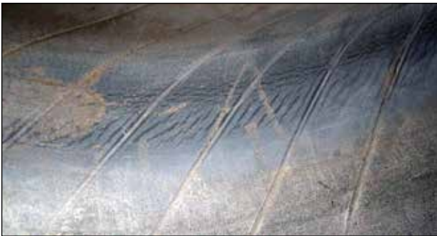
EFFECT: Inner Liner Marbling – Creasing CAUSE: Underinflation
