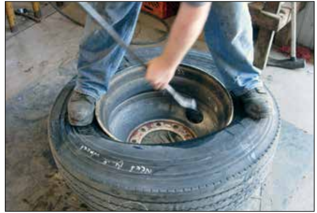
8 Mount second bead using same method.
