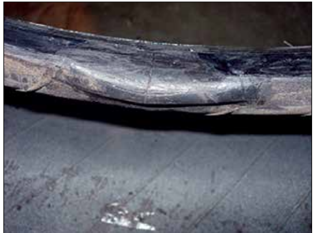
Bad Bead Repair
