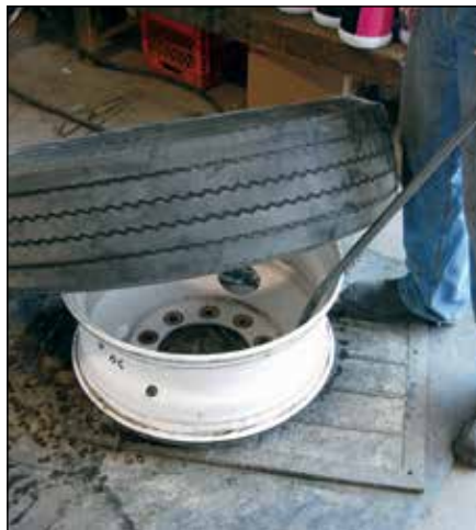
10 Allow the assembly to drop, and rock the tire from the wheel.
