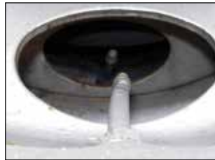
Incorrect Dual Wheel Placement
