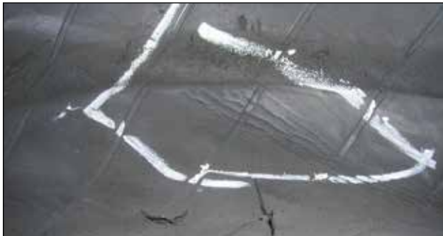
Inner Liner Marbling/Creasing
