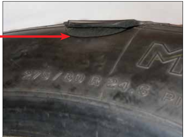
EFFECT: Sidewall Separation Due to Air Infiltration CAUSE: Improper Repair
