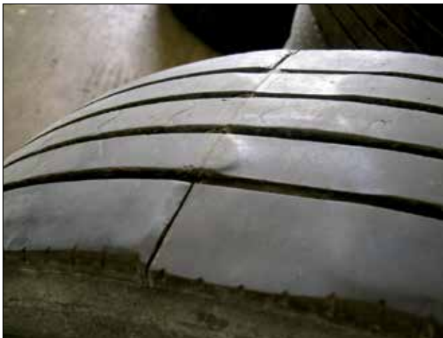
Open Splice Joint
