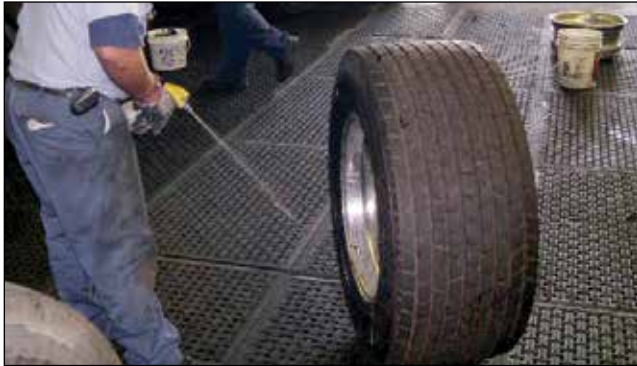
Lubricating Beads for Dismount
