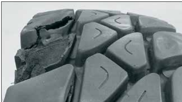
Exceeding speed rating for on/off road tires may cause premature or sudden tire failure.
