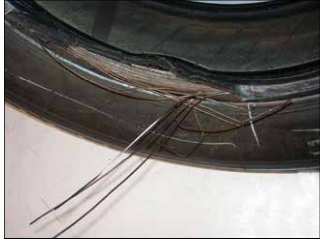
EFFECT: Bead Turning, Cracking/Splitting, Unwrapping from Heat CAUSE: Excessive Heat
