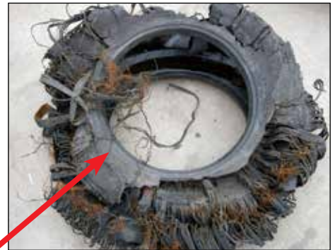
EFFECT: Crown/Sidewall Injury Resulting in Tire Pressure Loss CAUSE: Nail Hole Bolt/Debris Penetrating the Liner
