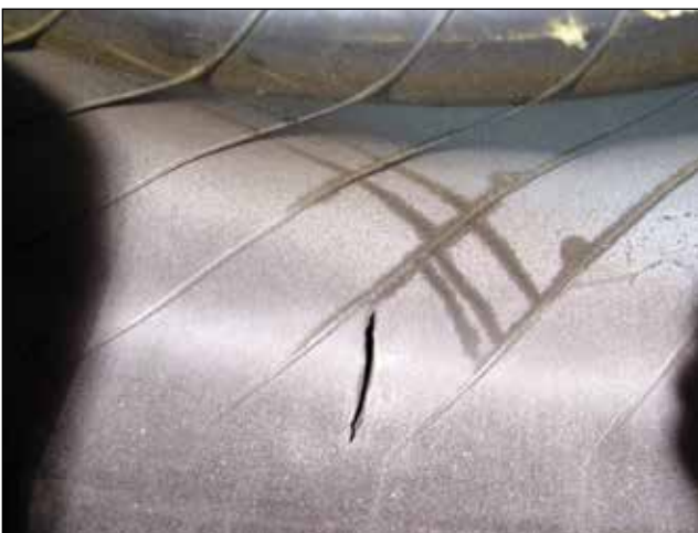
EFFECT: Inner Liner Split CAUSE: Sidewall Impact
