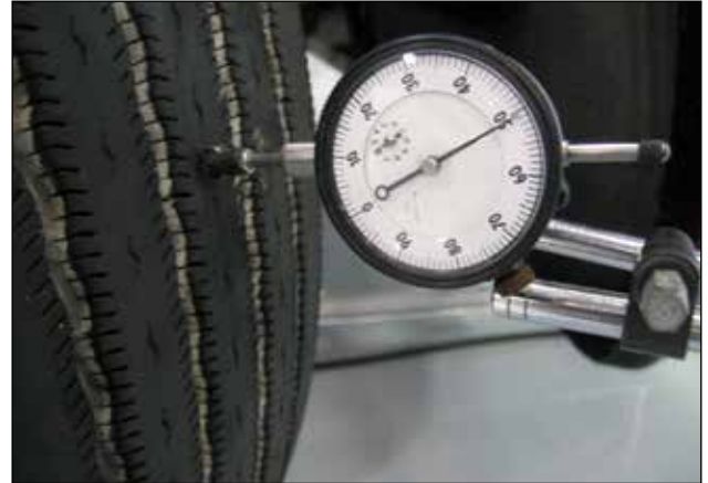
Measuring Radial Runout on Center Rib
