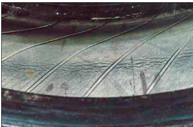
Potential Zipper Rupture
