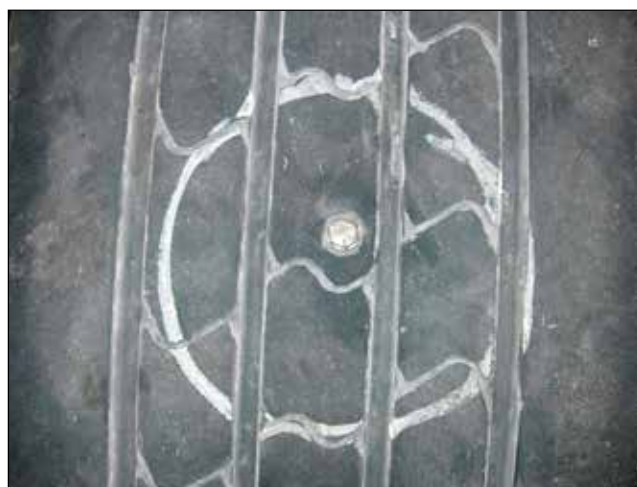
EFFECT: Object that Penetrates into the Tire and Through the Inner Liner CAUSE: Nail, Bolt, Screw, etc.
