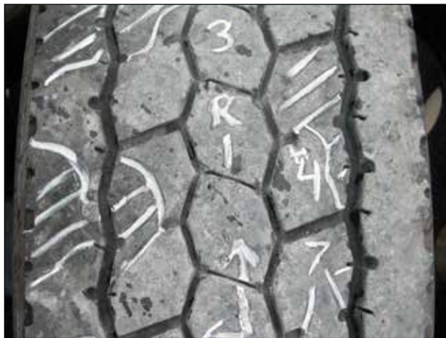
Cupping Wear – Drive
