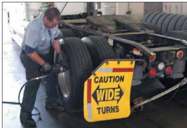
Mounting Dual on the Vehicle
