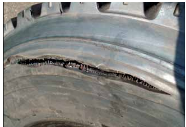
Zipper Resulting from Run Flat Condition
