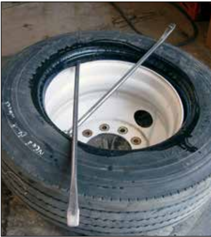
7 Completely unseat the first bead.
