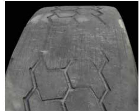
Brake Skid Damage
