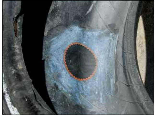
Improper Repair, Tube Repair Patch in Radial Tire, and Bead Damage from Demounting
