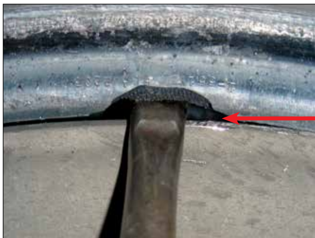
EFFECT: Bead Area or Inner Liner Damage CAUSE: Improper Demounting Procedure, Lack of Lubricant
