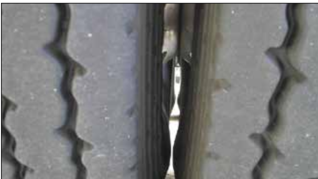
EFFECT: Friction Severely Weakens the Casing CAUSE: Improper Minimum Dual Spacing
