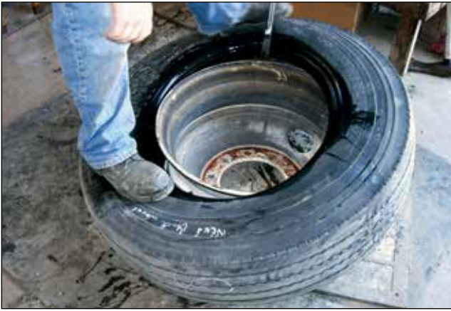
7 If necessary, continue to work the first bead on with proper tubeless tire tools like T45A tire iron.
