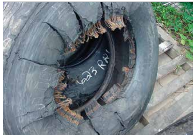
3rd Stage – Complete Unwrapping of the Casing Ply
