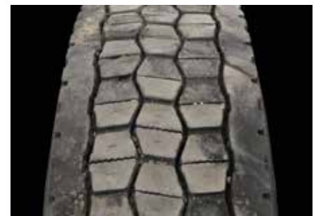
Cupping / Scallop / Alternate Lug Wear
