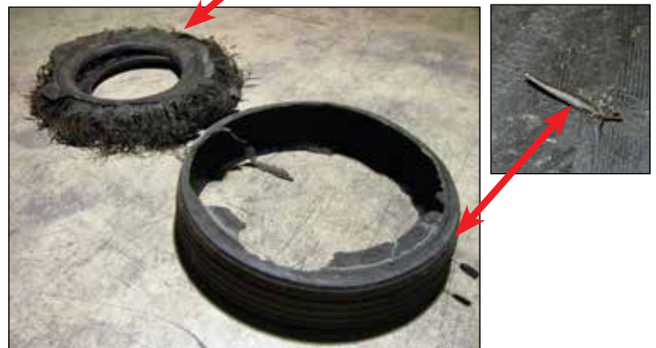
EFFECT: Run Flat CAUSE: Crown Perforation/Penetration
