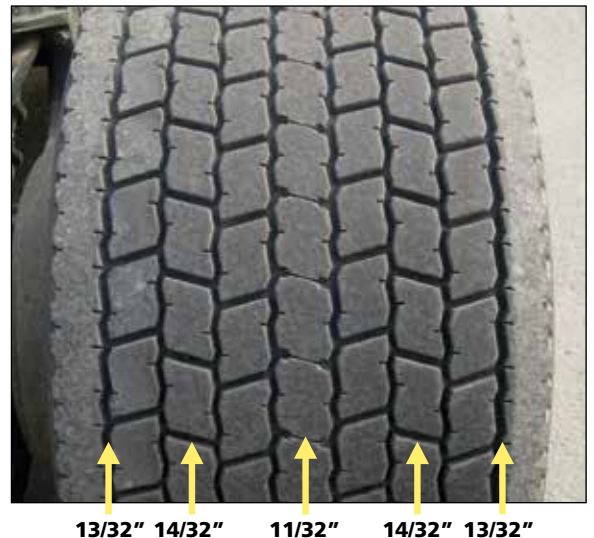
Inset: Notice appearance of shoulder-scrub on side of tread-blocks inner/outer shoulders.
