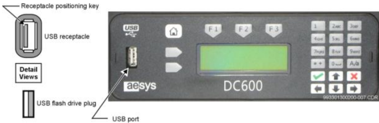
Fig.8.4 — DC600 Flash Drive Location and Connection Receptacle
