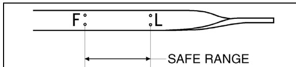
ENGINE OIL LEVEL DIPSTICK
