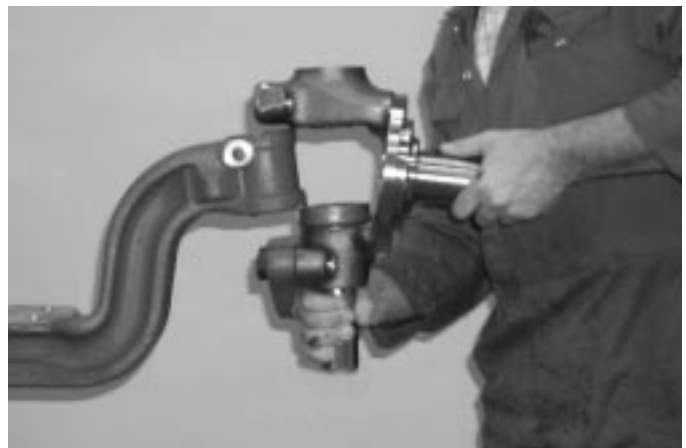
TOP OF THRUST BEARING NOTE DIRT SEAL
