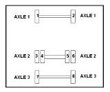
The sequence increments to the next wheel on the same axle counting wheels from left to right and then moves to the next axle counting axles from front to rear. The display activates the next wheel parameter each time a wheel is done. This parameter is use by the vehicle electronic to activate an audible signal on the vehicle thus providing a feedback to the user that he can move to the next wheel.
