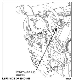
The automatic transmission oil level dipstick is accessible through the engine compartment rear door and is located on the left side of the engine.
