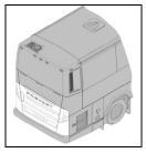
То open engine compartment door, first open engine compartment curbside door. Lift the latch release lever, place hand on the upper right of the rear door and pull rearward.
