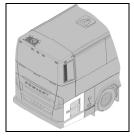
Lock this door using the exterior compartment key. Lift up protector cover to gain access to the lock. Pull up the door handle to release the latch and then pull the door open.
