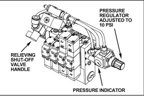
INFLATABLE SEAL RELIEVING SHUT-OFF VALVE 26098
