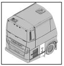
To unlock the main power compartment door, use the exterior compartment door key. The door will pop open.
