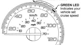
EXAMPLE OF THE SPEEDOMETER LED DISPLAY WHEN THE FORWARD VEHICLE IS SLOWER WHILE THE COACH TRAVELS WITH THE ACB CRUISE CONTROL ON AND SET 06729\_3
