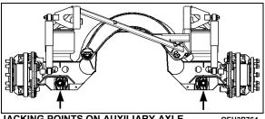
JACKING POINTS ON AUXILIARY AXLE
