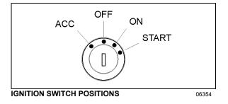
The ignition switch is located on the lower left side of the dashboard. It has four positions:
