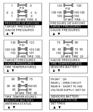
The display remains in this mode with the menus appearing at the bottom until the pre-trip check sequence starts again.
