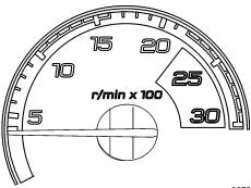
Tachometer (rpm x 100)
