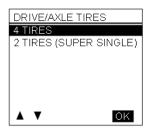
Pressing the up down arrow when the number of tires is highlighted allows flipping the number to 2 or 4 which are the only valid choices.
