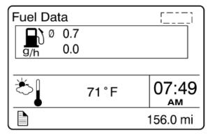
The outside air temperature, fuel flow and the odometer are part of the default display. You can change the default display by your selection of favorite gauges using the Driver Information Display sub-menu Favorite Display Setting. Refer to *Other Features* chapter for more information.
