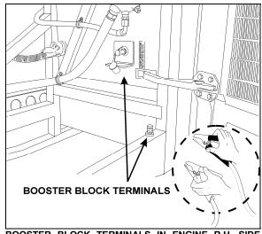
BOOSTER BLOCK TERMINALS IN ENGINE R.H. SIDE ACCESS COMPARTMENT 18645
