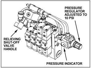
INFLATABLE SEAL RELIEVING SHUT-OFF VALVE 26098
