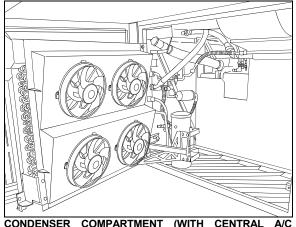
CONDENSER COMPARTMENT (WITH CENTRAL SYSTEM, DEF TANK NOT SHOWN)
