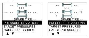
As illustrated, the pressure readings will appear replacing the dash lines as the TPMS display starts to receive pressure data from the TPMS receiver. It can take 1 minute to get all pressure readings updated since the sensors transmit at a one minute interval.
