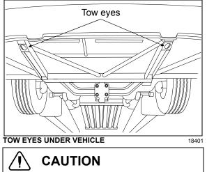
Make sure axle shafts or driveshaft are installed correctly after towing. Tighten axle shaft and driveshaft nuts to the correct torque settings. Do not invert shafts.
