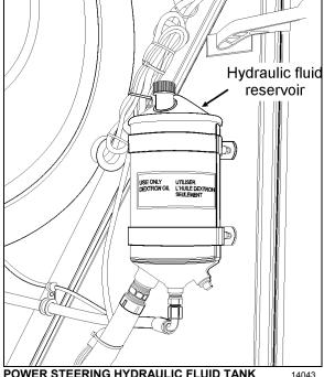
POWER STEERING HYDRAULIC FLUID TANK
