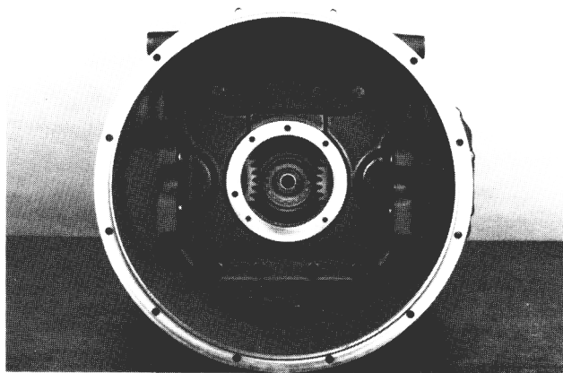
7. Remove the input bearing cap, gasket and input shaft,
