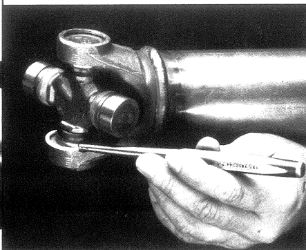
Removing an inside snap ring.
