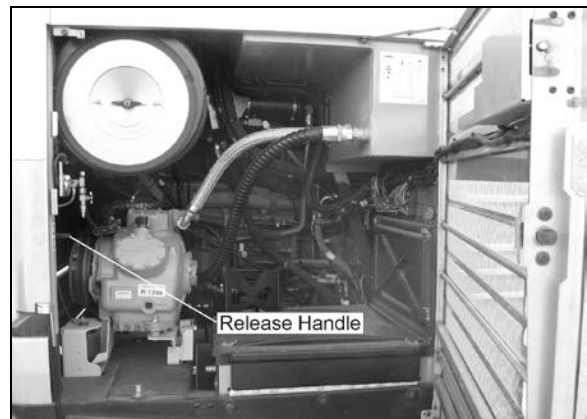
OPENING THE ENGINE COMPARTMENT REAR DOORS FROM R.H. SIDE DOOR 18547
