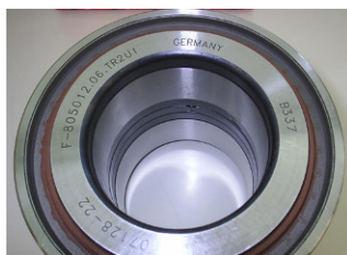
Bearing oil side. There isn't any place to fit the o-ring.
