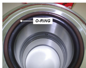
Bearing air side. It can be seen the o-ring (brown component) installed
