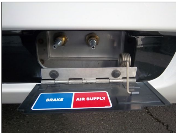
QUICK CONNECTOR FITTINGS ON FRONT BUMPER
